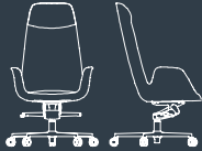
HALIA S0 EXCTV 5SB/C/HA/5TM L: 745 mm / 29.3 inch D: 709 mm / 27.9 inch H: 1143-1228 mm / 45.0-48.3 inch
